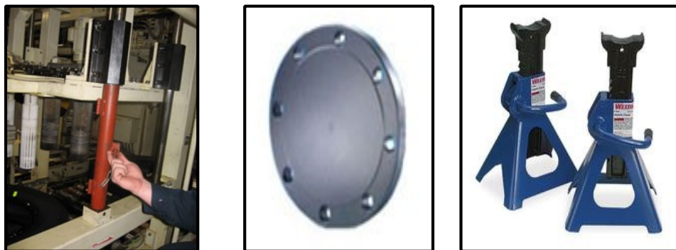
Blocking an Equipment Press, Pipe Blinding Flange, Support Stands used for Blocks
